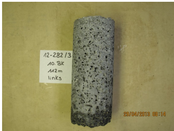
Abb. 32: Bohrkern CEM II/B-S 52,5R
