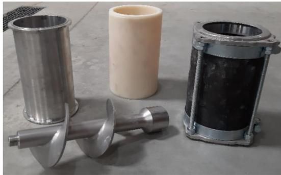
Links: X5CrNi18-10; Mitte: PA 6; Rechts: Schlauch Typ E592-EPDM
